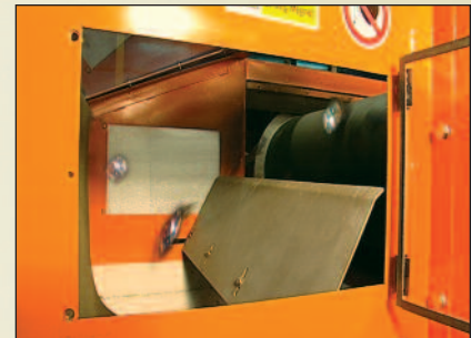
The RevX-E's powerful, Rare Earth magnetic rotor is ideal for recovery of valuable nonferrous metals in ASR, cullet, plastics, secondary metals and incineration ash applications.
