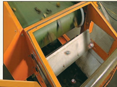
The RevX-E's powerful, Rare Earth magnetic rotor is ideal for recovery of valuable nonferrous metals in ASR, cullet, plastics, secondary metals and incineration ash applications.
